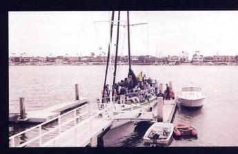
SAFETY: This photo shows a 65 undergoing Coast Guard stability testing, using a small army (50 people) as moveable ballast. Notice that the waterline stripe is still visible, even with this excessive load.
