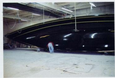
This is the mold from which the 65 hull is produced. It will be polished and waxed. The white exterior hull finish will be sprayed on the mold, followed by many layers of hand laid fiberglass mat and woven roving. Each layer is impregnated with resin and cured.
