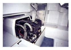
This shows the front cover in place. You still have access to most of the items on the engine that may require attention. The front cover seldom comes off. (It take about 10 seconds to remove each cover.)
