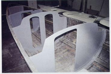
This picture shows the transverse bulkheads that support the hull stringers and hull shell. These bulkheads are bonded on both sides to the shell and stringers with 1/4" thick fiberglass layups. Few boats have this many full bulkheads, and they give the hull tremendous stiffness and strength.
