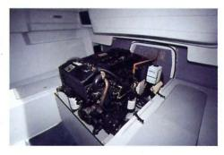
This photo shows the engine with both of its soundproofed covers removed. This is the compartment aft of the watertight bulkhead. As you can see, every part of the engine is completely exposed.
