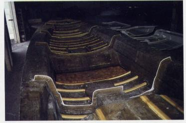
This is the upside down deck, without the cosmetic liners that form the ceiling. You can see the stringers that give the deck its stiffness, and the partial bulkheads that bolt securely to the tops of the hull bulkheads. We use heavy, solid laminates rather than low density cored construction for strength and stiffness.
