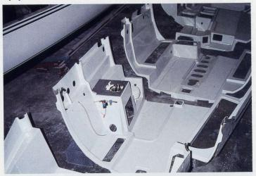
These are the individual fiberglass liners that fit between the bulkheads. These form the floors, berths, seats and interior cabinetry. Each liner is produced on its own mold. These liners bond to the hull and bolt to the bulkheads and add a great deal to the structural integrity of the boat.
